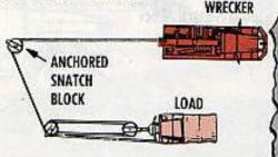
Move everything and everyone out of the angled area when the cables are under stress. Cables have been known to snap. And when that happens the cable's deadly whiplash can easily slice through humans, trees, equipment, and anything else within its reach. So pick a spot at least as far away as the length of the paid-out cable for any on-lookers or any baggage you may've had to unload.
