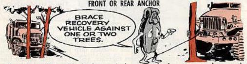
If you're pulling with the front winch you can back up to a good tree and tie the truck's pintle hook to the tree. Or, brace the front, or the rear, of your recovery vehicle against one or two trees for a front, or rear, winching job.
