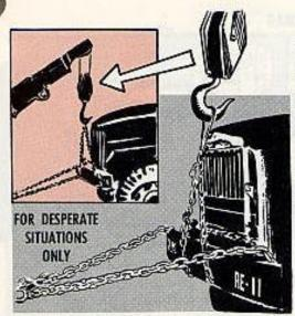
Use two log chains. Put one chain around the bumper of the dead truck, and then through the wrecker's pintle hook. Wrap the other chain around the truck's bumper and then up to the wrecker's hook.
