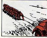
When you're without trustworthy mechanical power, 15 to 20 men on a rope provide a hefty pull. Put all the men on one side of the rope, and keep the line from under-foot. To give the men a 2-to-1 advantage anchor one end of the rope in line with the load. Attach a single snatch block to the load. Run the rope from the anchor through the block and to the men.
