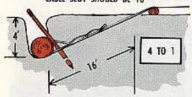
Sink a strong log in a deep trench, and tie on to it. You need a T-shaped trench, and the softer the ground the deeper the trench should be. Make the wall which will take the pull slant away from the load. The leg of the T is an upward slanting slot to take the cable. And the longer and deeper the slot the straighter and stronger the pull will be on the log.
