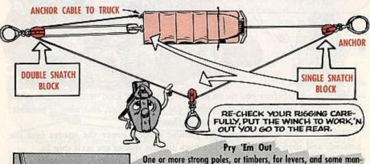
One or more strong poles, or timbers, for levers, and some manpower can pry out a truck that's gone head-first into a narrow ditch.
