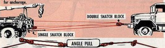
When you can't set-up your recovery power for a straight pull on the load, you have to line-up an especially good anchor in the direction the load must move, and find the best possible stand for your wrecker, and anchor it there dig in the rear spades, and anchor it by its front winch, if need be.
