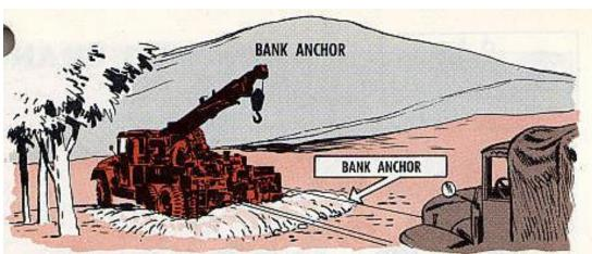
When your wrecker is sitting on hard ground (but, off the road) you can dig in its rear wheels for holding power. Make a straight embankment across the rear to block the pull, and fix a slight ramp in front to let you back in and pull out easy like.
